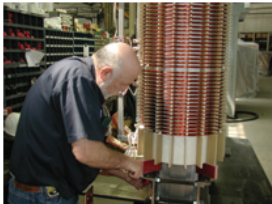
Dry type transformer for emergency replacement - designed to duplicate 'form, fit and function' as closely as possible
