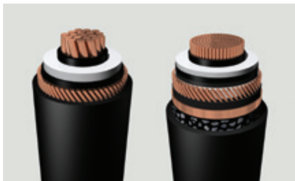
Figure on left is typical construction of a medium-voltage underground cable utilizing TR-XLPE solid insulation. Figure on right is typical construction of a high-voltage underground cable with PE-based jacketing and semiconductive layers and super-clean XLPE solid insulation.
